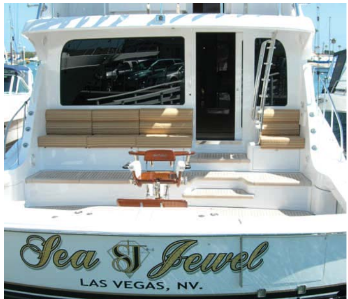
This 68 has a low-slung transom that begs to be backed down, a tank capable of holding 100 mackerel, and the ability to hold six tuna.
