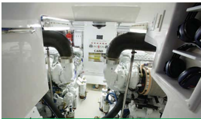
Two MAN V-12s with plenty of room on all sides for servicing.
